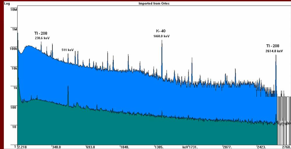
•Fig.2. Background spectra of bare big volume Ge detector ( upper spectrum) and shielded detector (lower spectrum )
