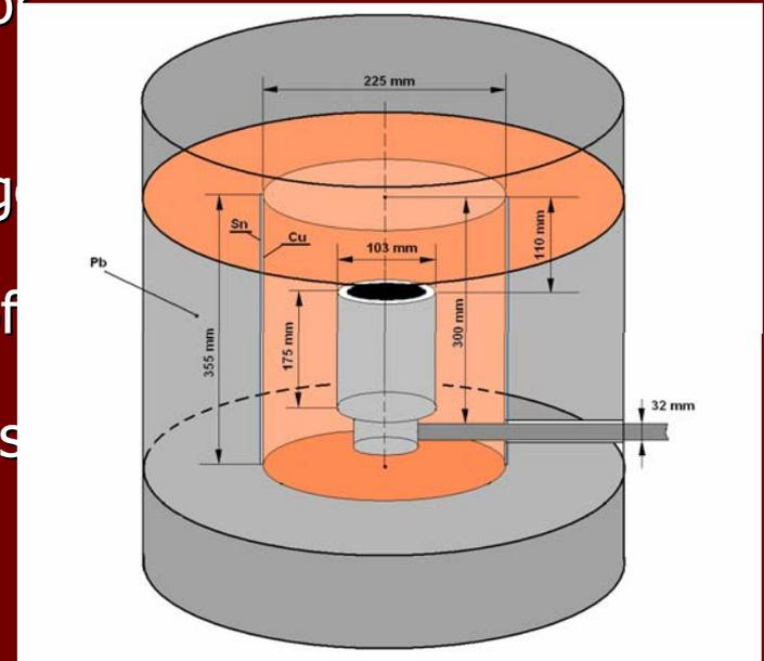
*Fig 1b. Position of the detector housing inside lead shield*
