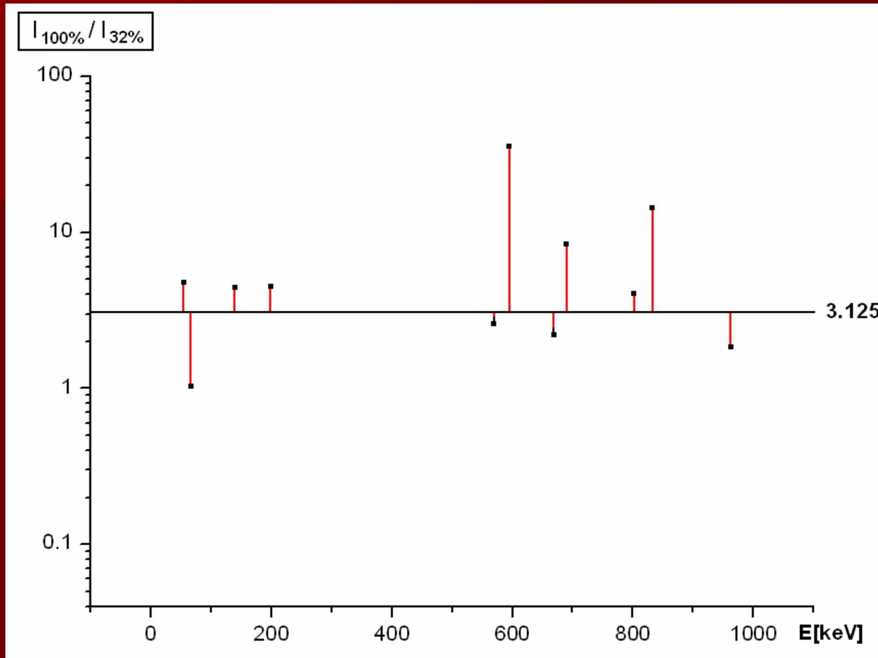
*Fig.4. The ratio of intensities of neutron induced lines in 100% relative efficiency Ge detector and 32% relative efficiency Ge detector ,respectively . Value 3.125 is the ratio of relative efficiencies for two detectors.*
